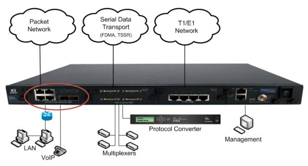
The Ethernet Interface Option Module takes Ethernet-based applications into the PA iQ and provides the network connection for converged Ethernet and Serial application streams across a Packet-based transport network
